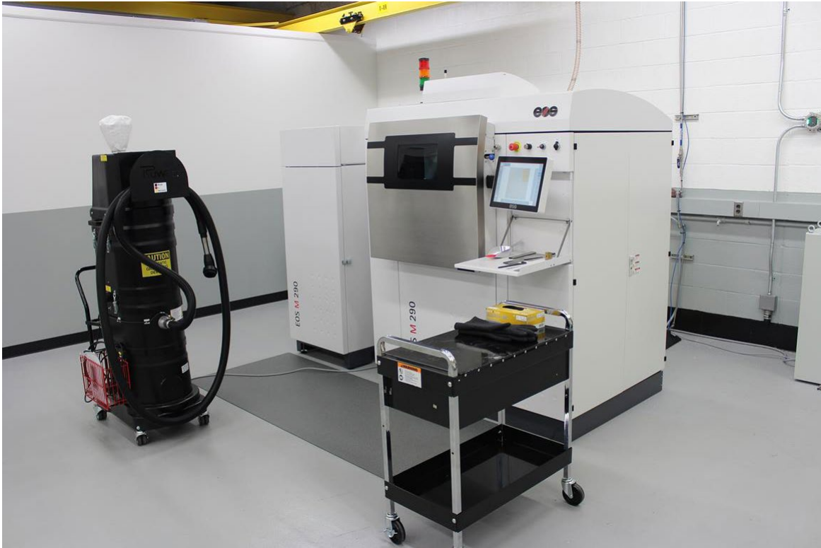
EOS M290 located at our Cabot manufacturing campus.
